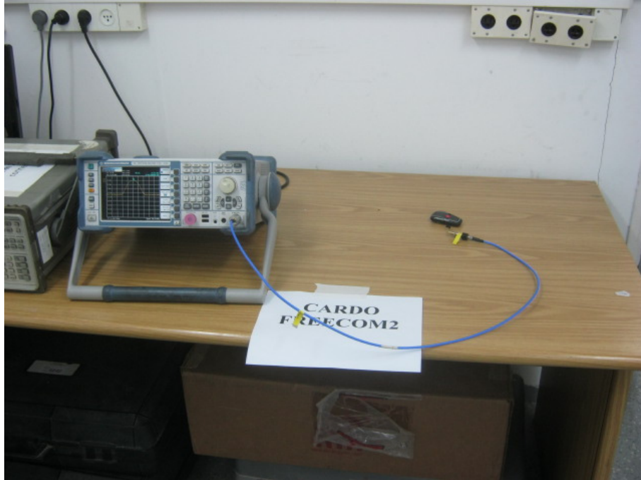
Figure 5. Conducted Emission From Antenna Ports Test Set-Up
