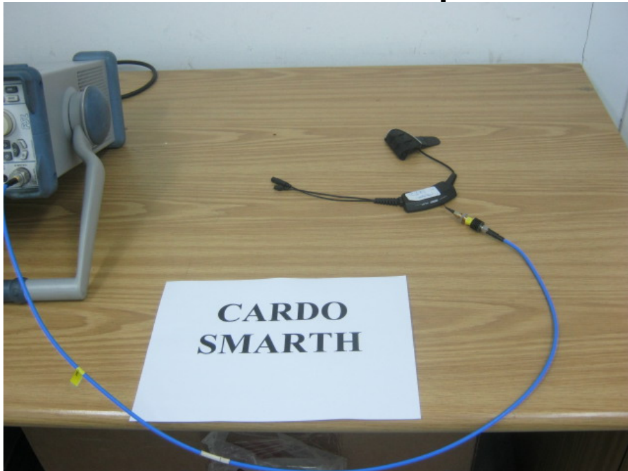
Figure 5. Conducted Emission From Antenna Ports Test
