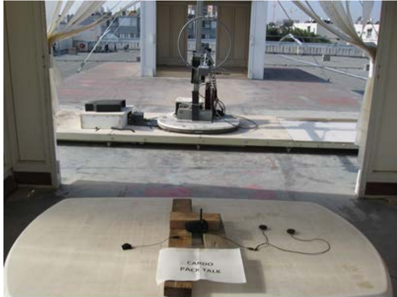
Figure 2. Radiated Emission Test
