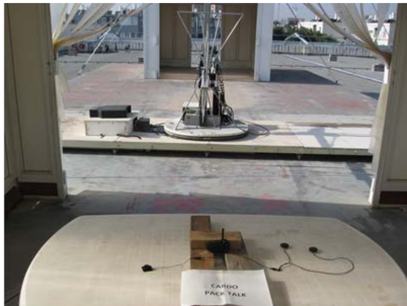
Figure 3. Radiated Emission Test
