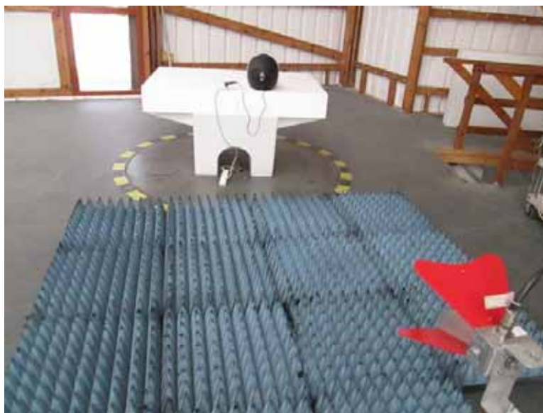
Photograph 8.2.3 Setup for final radiated emission measurements, EUT cabling
