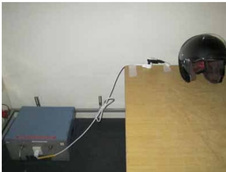
Photograph 8.1.1 Setup for conducted emission measurements
