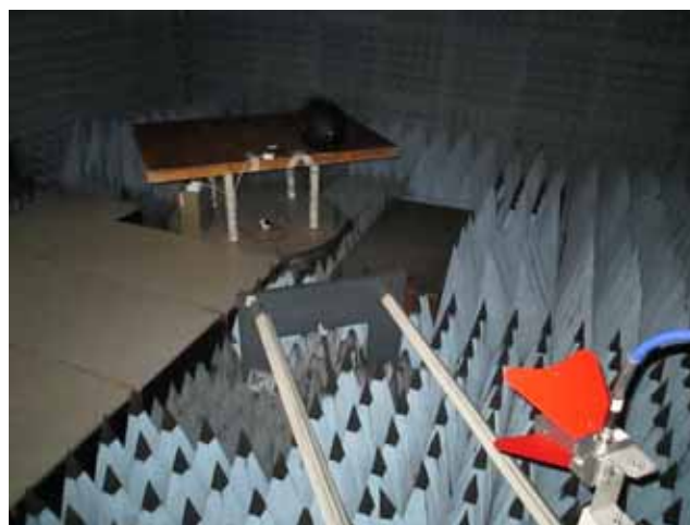
Photograph 8.2.1 Setup for radiated emission measurements
