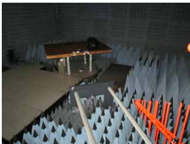
Photograph 8.2.1 Setup for radiated emission measurements
