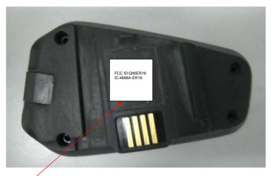
Label with FCC ID:Q95ER16 and IC:4668A-ER16 will be located at the rear side panel.
