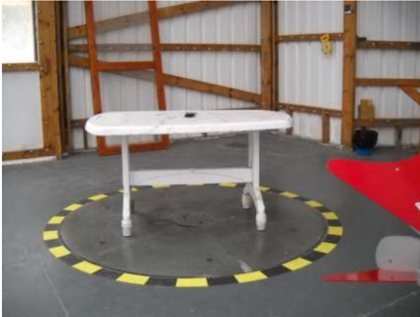
Photograph No.4 Spurious emissions field strength measurement setup at the OATS
