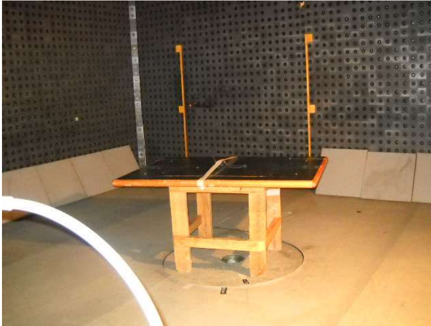
Photograph No.1 Spurious emissions field strength measurement setup in the anechoic chamber below 30 MHz
