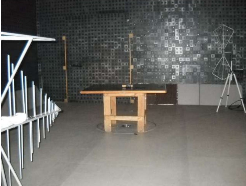
Photograph No.2 Spurious emissions field strength measurement setup in the anechoic chamber in 30 - 1000 MHz
