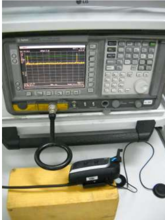
Photograph No.5 Occupied bandwidth, carrier frequency separation, number of hopping frequencies, average time of occupancy measurement setup
