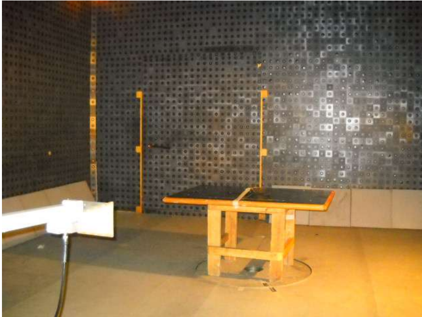
Photograph No.3 Carrier and spurious emissions field strength measurement setup in the anechoic chamber
