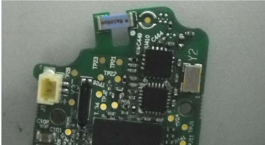
Photograph No.7 Bluetooth headset antenna for operation at 2401 MHz
