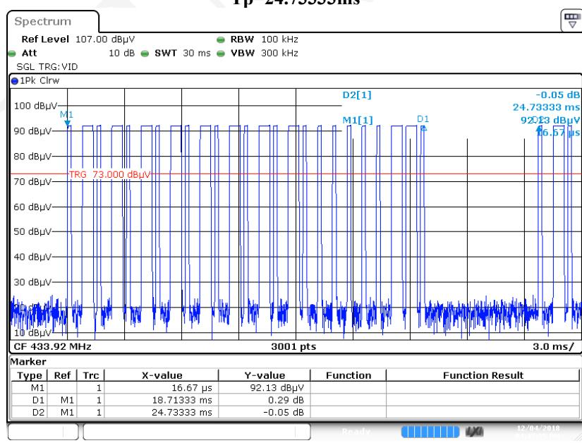
**Duty Cycle Burst 1**
