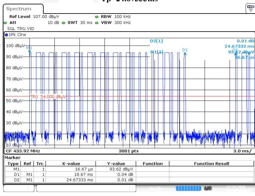
**Duty Cycle Burst 1**
