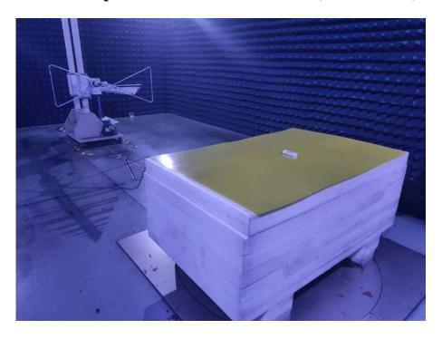
**Radiated Spurious Emissions Test View (Above 1GHz)**
