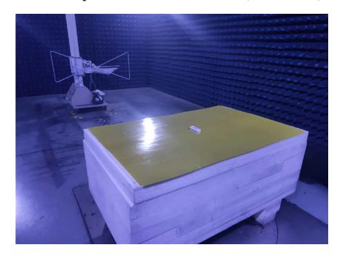
**Radiated Spurious Emissions Test View (Above 1GHz)**
