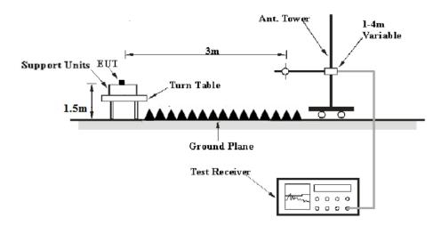
The radiated emission tests were performed in the 3 meters test site, using the setup accordance with the ANSI C63.10 - 2013. The specification used was the FCC 15  $\S$  15.205, 15.205 and 15.231.
