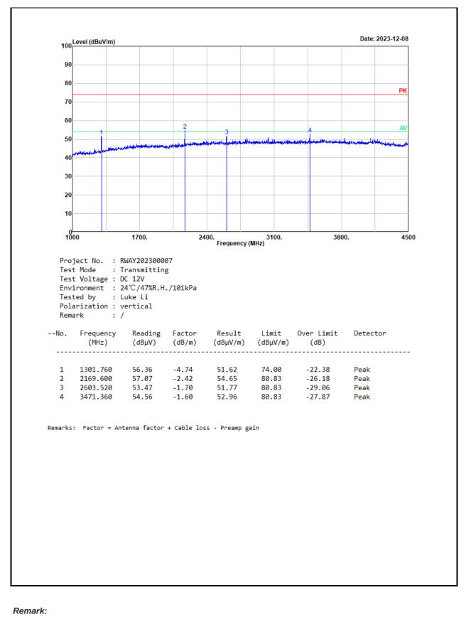
Level = Reading + Factor Factor = Antenna factor + Cable loss – Amplifier gain Over Limit = Level – Limit
