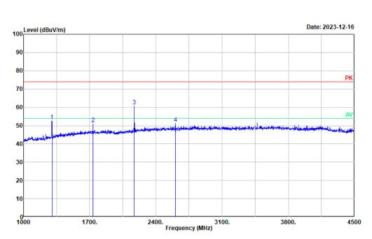
Project No. : RWAY202300009 EUT/Model No.: BH-20E Test Mode : Transmitting Test Voltage : DC 12V
