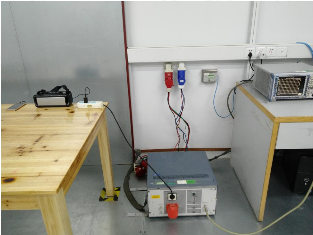
RADIATED EMISSION TEST SETUP BELOW 1GHZ
