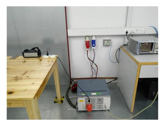
RADIATED EMISSION TEST SETUP BELOW 1GHZ
