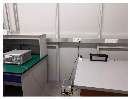
FCC RADIATED EMISSION TEST SETUP
