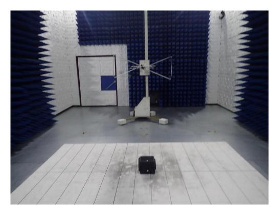
RADIATED EMISSION TEST SETUP ABOVE 1GHZ
