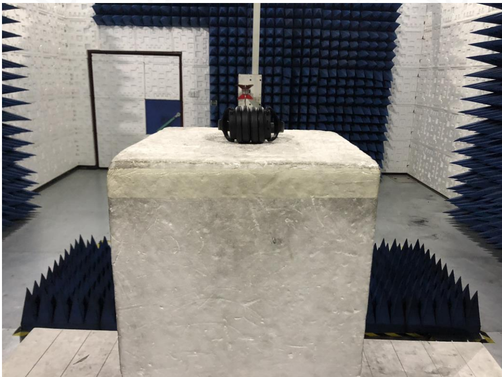
RADIATED EMISSION TEST SETUP ABOVE 1GHZ
