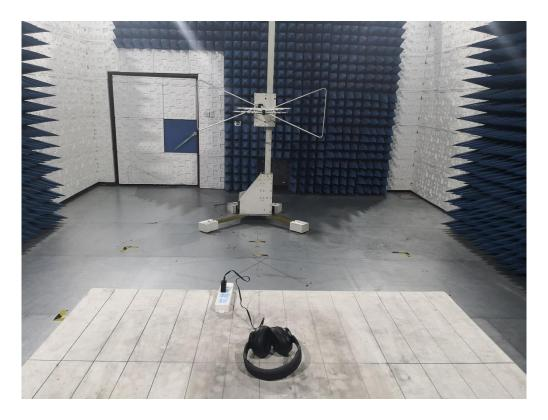
RADIATED EMISSION TEST SETUP ABOVE 1GHZ
