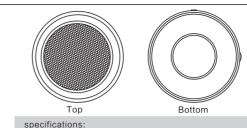
Power: 3W (Max) Battery voltage: 3.7V Battery capacity: 500mAH Battery charging voltage: 5v  $\pm$  0.25v Diameter of speaker: 40mm,4  $\Omega$ Frequency: 180Hz–20KHz S/N:  $\geq$ 80dB Working time: 2–5 hours Working Distance:10M(Distance vary with environment and Bluetooth devices) Compliance with Bluetooth 3.0 Support A2DPV 1.2 2
