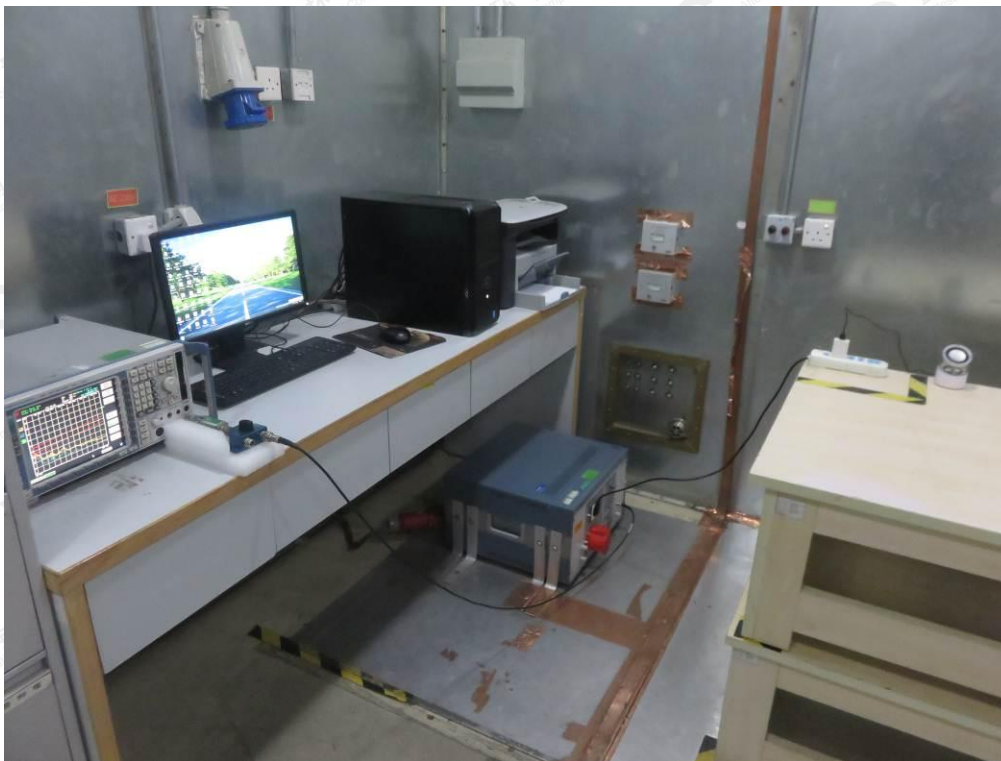
FCC RADIATED EMISSION TEST SETUP
