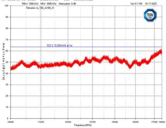
Note: testing was performed to 26.5 GHz, no emissions above 18 GHz were detected and the reading were below the applicable limit(s).
