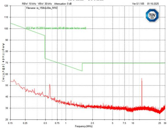
Note: Spike shown at 13.56 MHz is intentional RFID signal. Device was scanned down to 9 kHz, no emissions were detected below 150 kHz.
