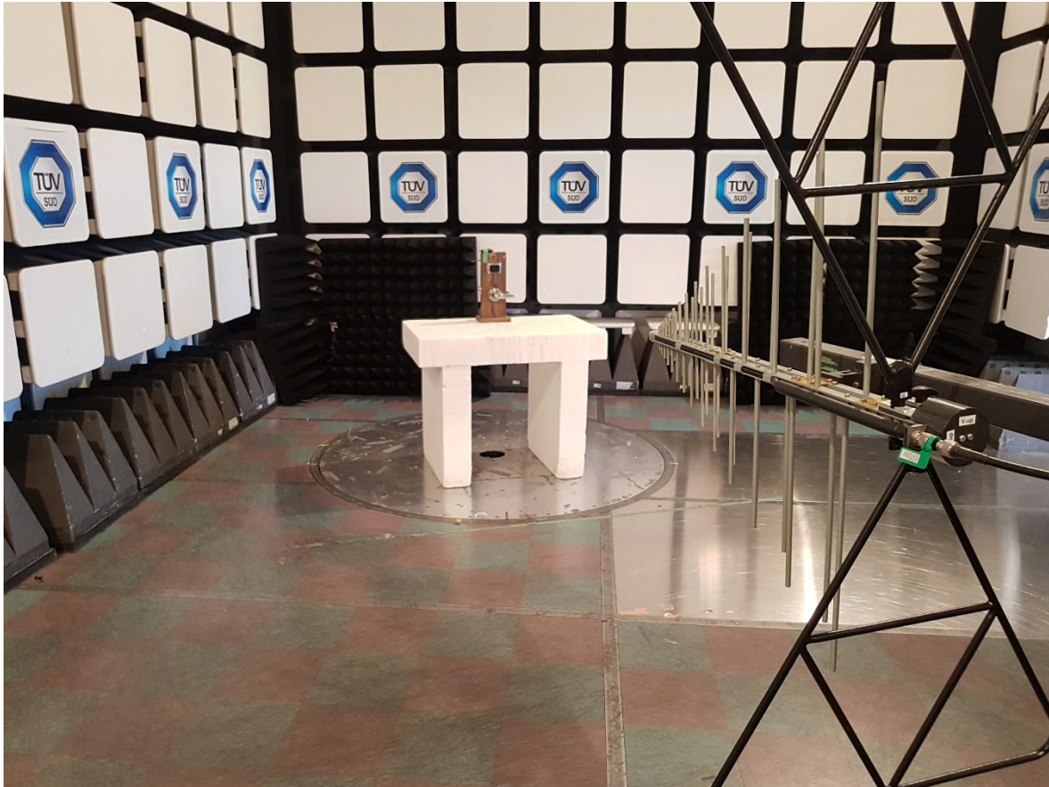
Figure 5 – Radiated Emissions Setup 30MHz to 1GHz
