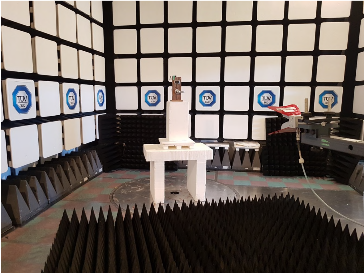
Figure 6 – Radiated Emissions Setup 1GHz to 4GHz
