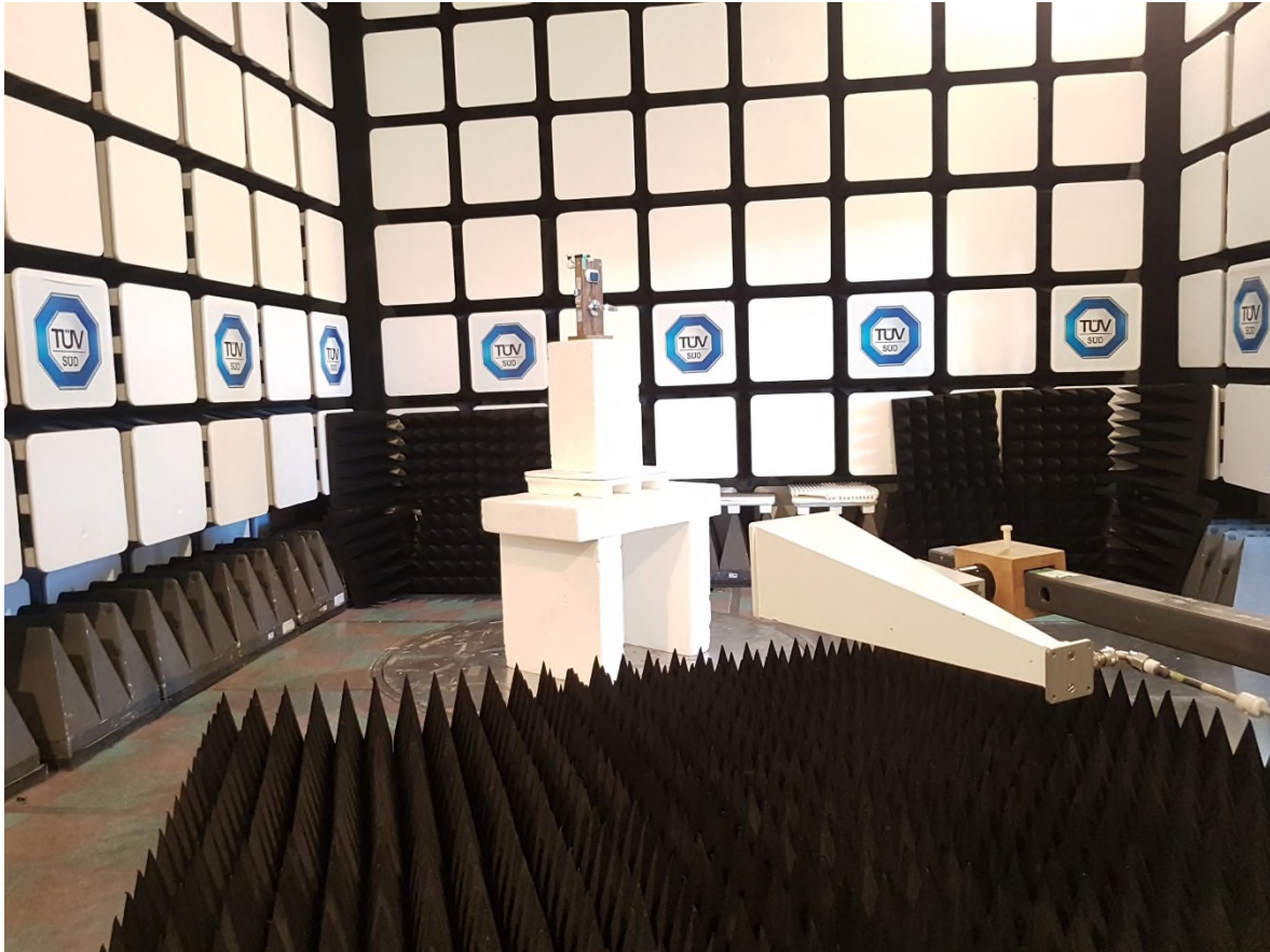
Figure 7 – Radiated Emissions Setup 4GHz to 18GHz
