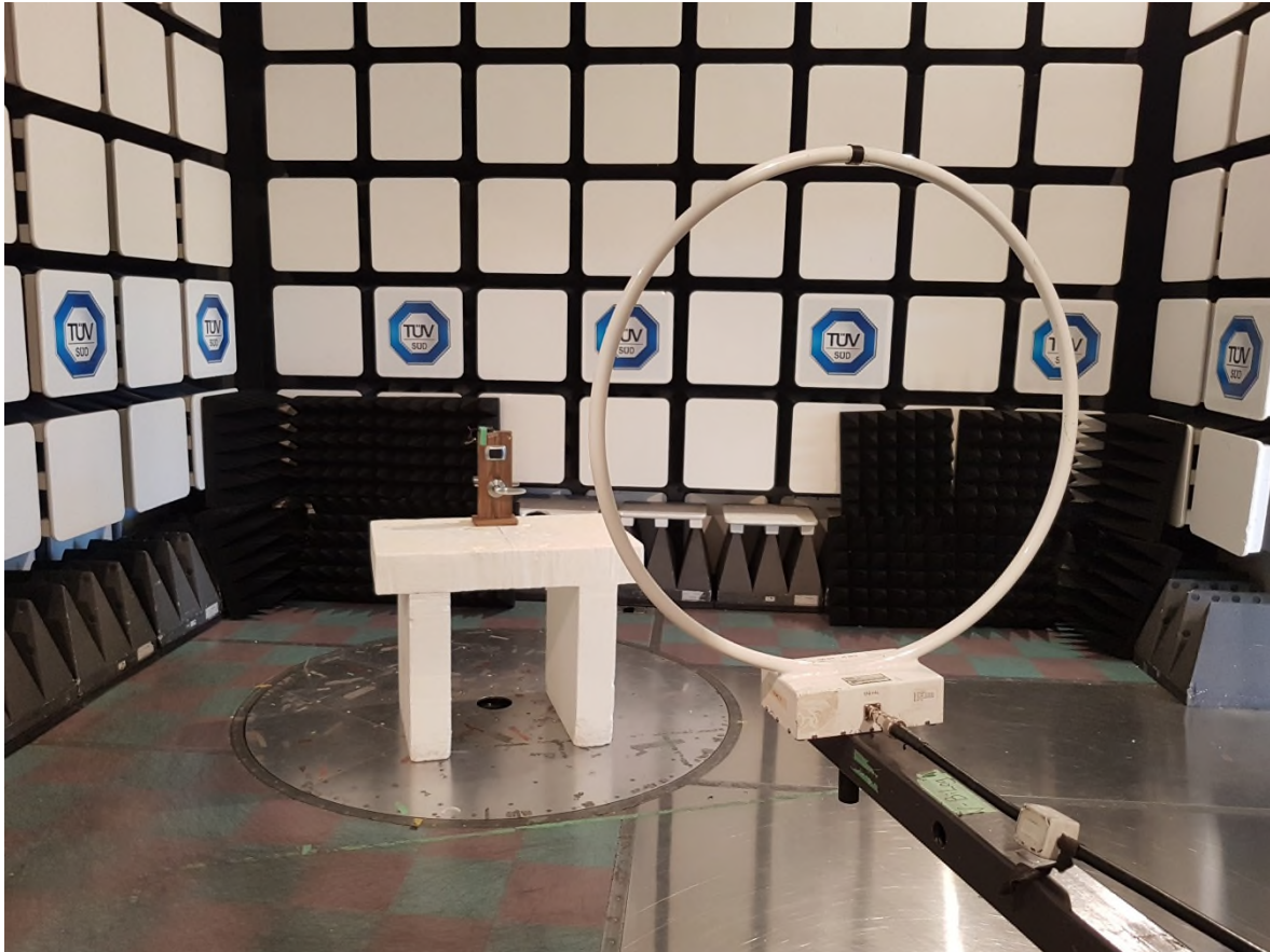
Figure 4 – Radiated Emissions Setup 9kHz to 30MHz
