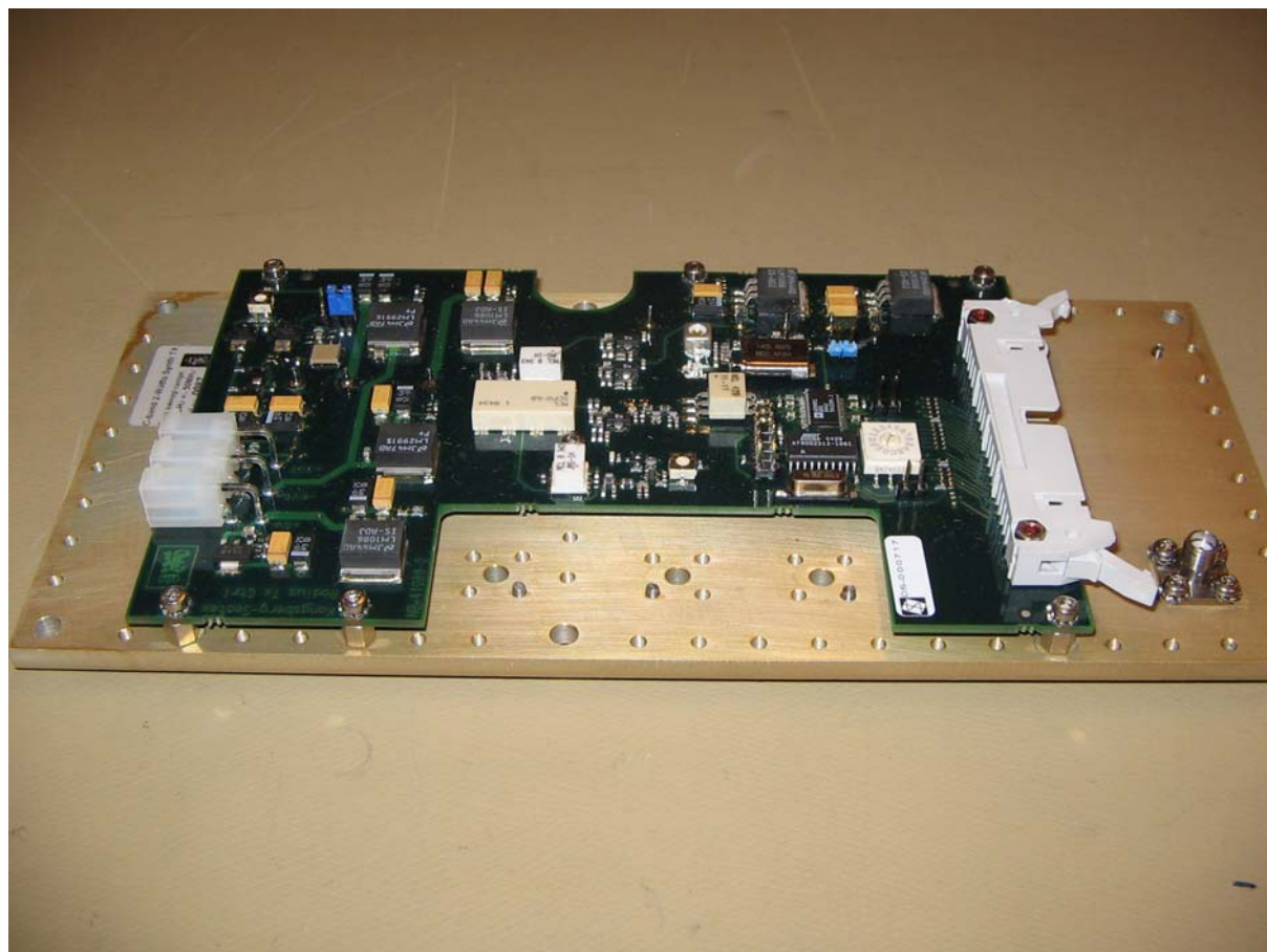
TX-CTRL board mounted on metal plate - interrogator
