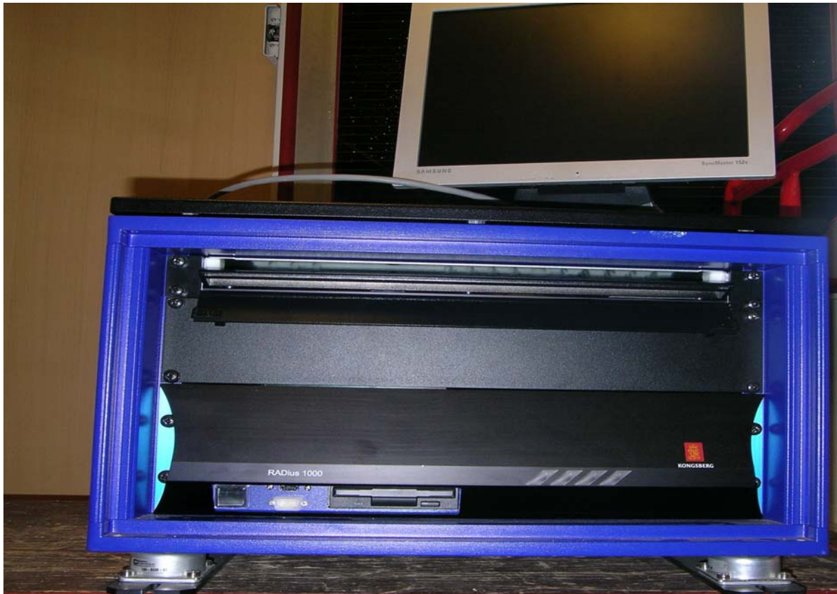
Industrial PC with screen to monitor and control the interrogator
