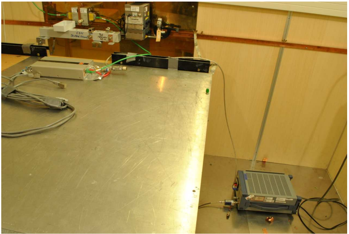
Notes: Test set-up for Conducted Emissions 10 kHz – 30 MHz
