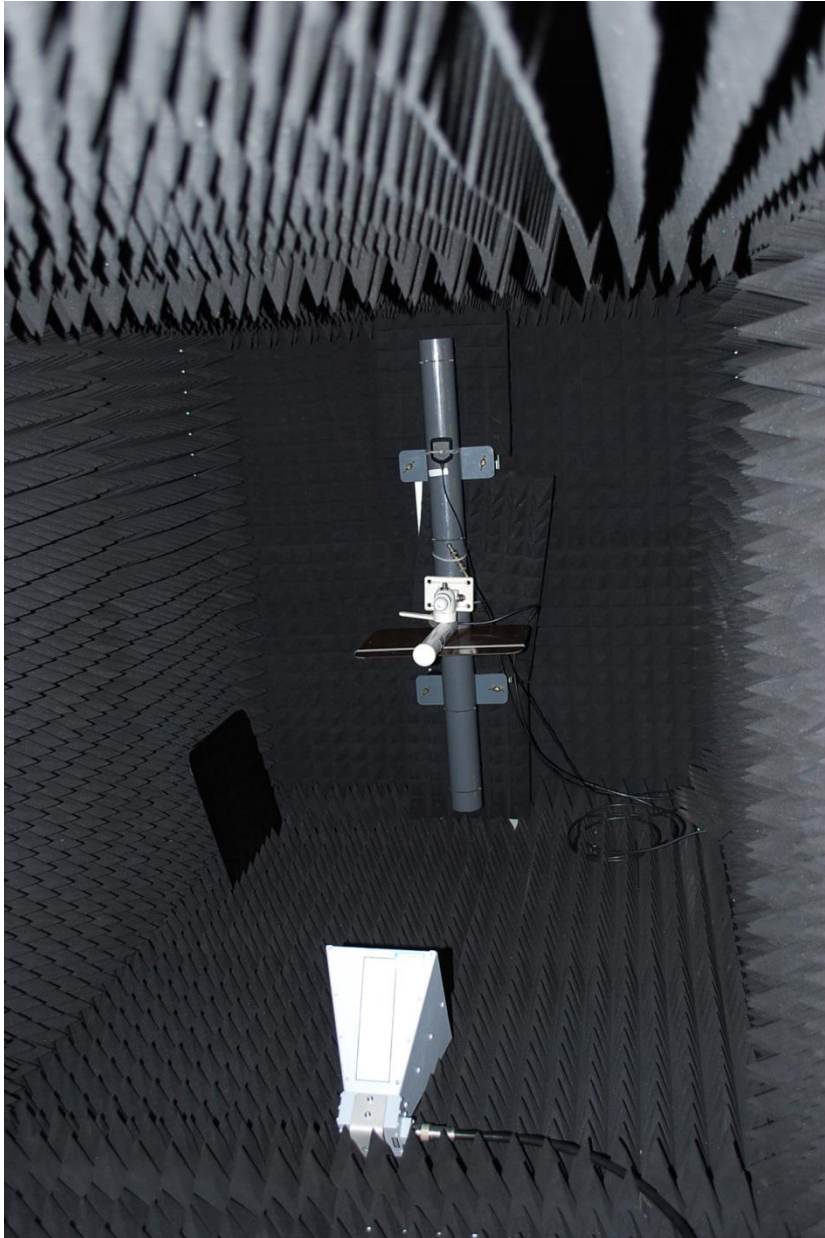
EUT antenna inside RF-Chamber
