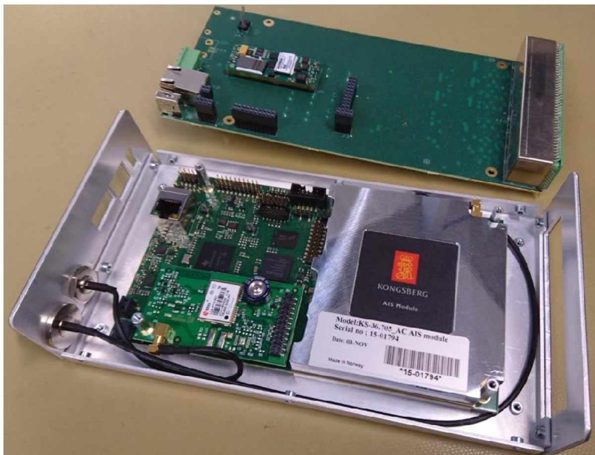
Figure 2 AIS 300 Main board with radio and rear of interface board - GPS receiver board on top
