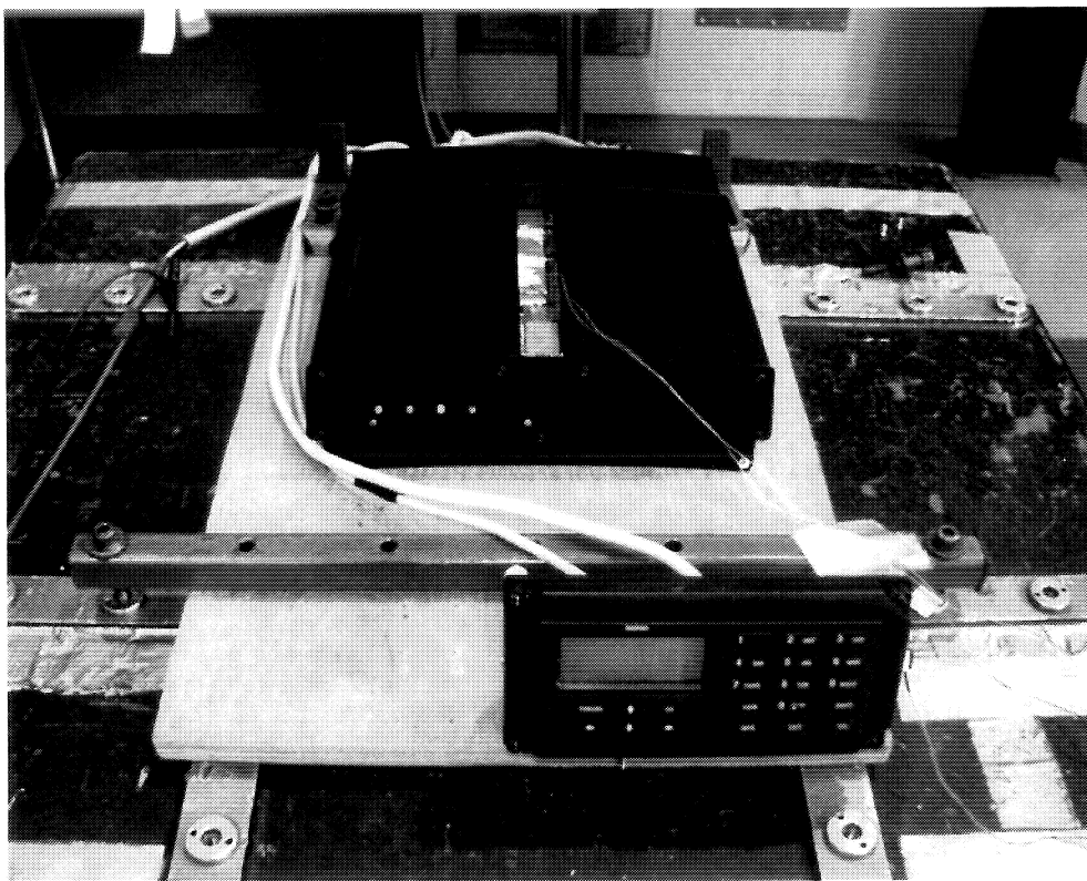
Mounting of EUT for vibration testing
