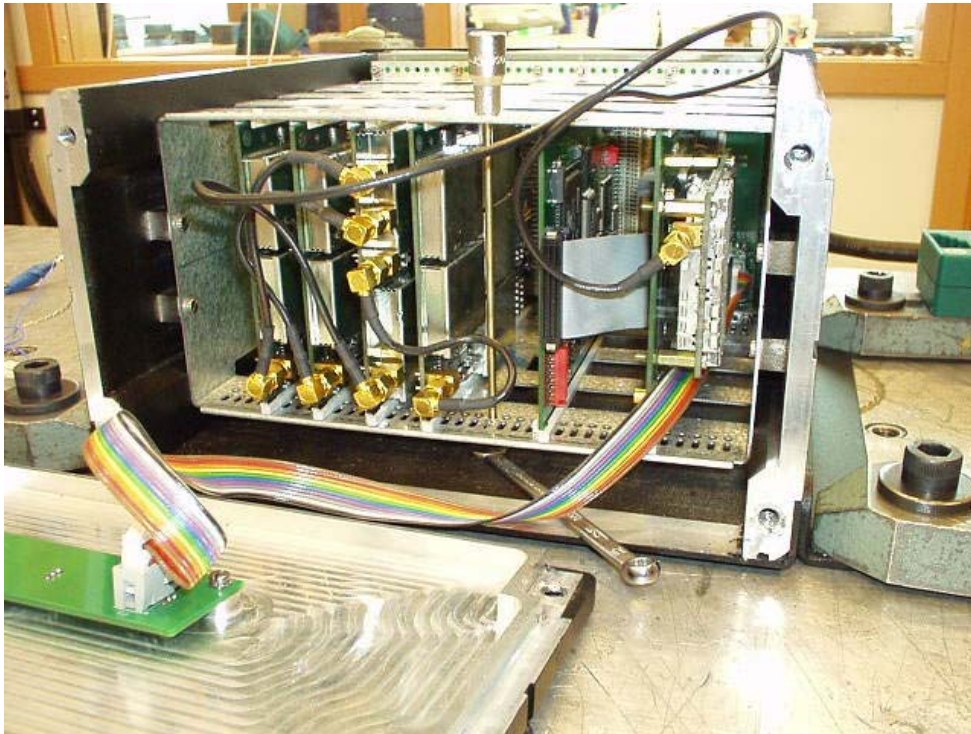
AIS main unit during resonance search test
