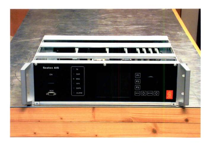
A modified Seatex AIS, Mainly used as a signal generator for the wanted signal
