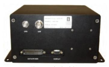
Figure 12 Rear side of mobile station
