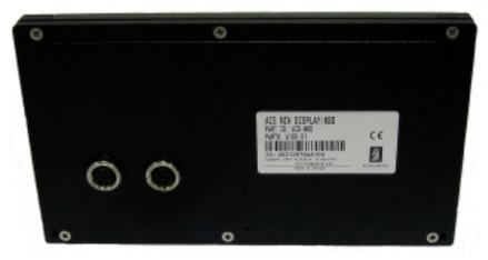
Figure 9 Rear side of the MKD unit and interconnection plug
