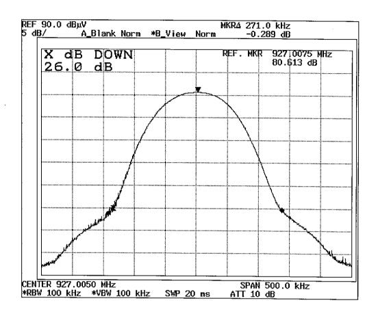
Frequency: 927MHz = -26dB Band width: 271kHz
