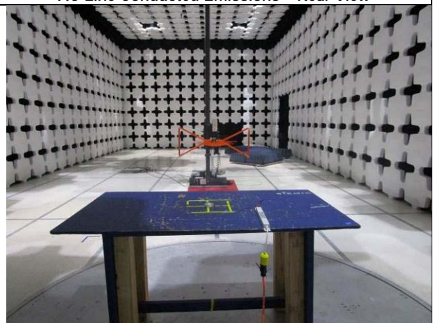
Radiated Emissions (<1GHz) – Rear View
