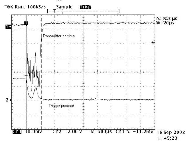
Plot showing transmitter on time. Note: To see Tx on time the button release is not seen.
