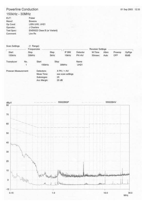
Receiver Mode Power Line Measurement
