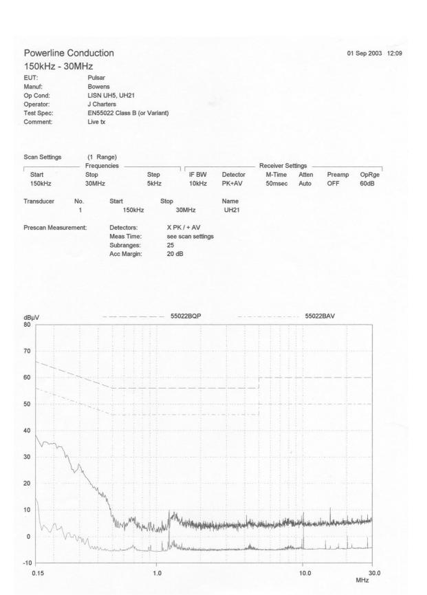
Transmitter Mode Power Line Measurement
