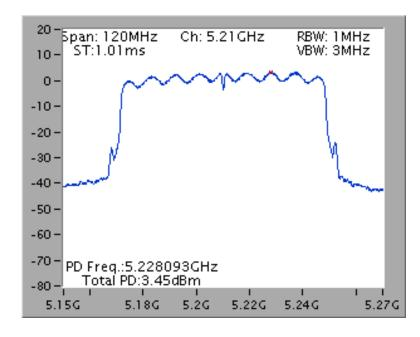
Power Density Plot on Configuration IEEE 802.11ac MCS0/Nss1 VHT80 / Chain 1 + Chain 2 / 5210 MHz
