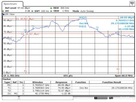
26dB Bandwidth and 99% Occupied Bandwidth Plot on Configuration IEEE 802.11a / Chain 1 + Chain 2 / 5785 MHz
