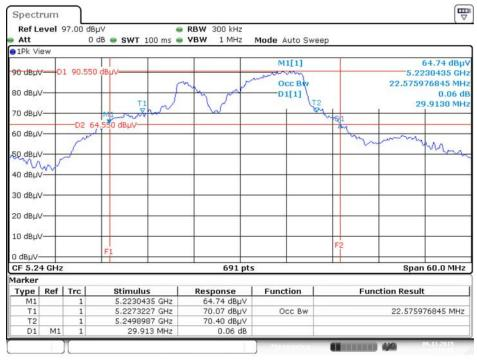
26dB Bandwidth and 99% Occupied Bandwidth Plot on Configuration IEEE 802.11a / Chain 1 + Chain 2 / 5240 MHz
