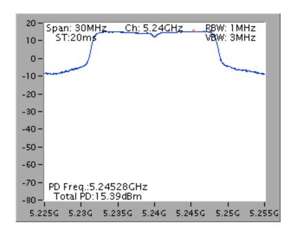
Power Density Plot on Configuration IEEE 802.11a / Chain 1 + Chain 2 / 5240 MHz
