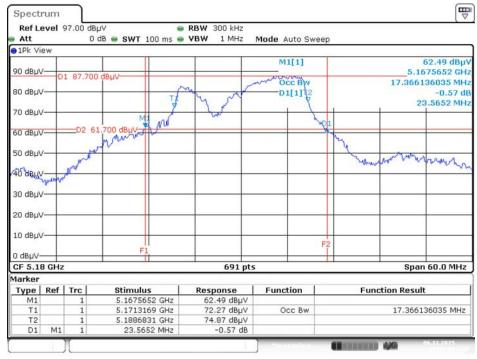
26dB Bandwidth and 99% Occupied Bandwidth Plot on Configuration IEEE 802.11a / Chain 1 + Chain 2 / 5180 MHz
