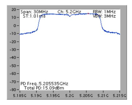
Power Density Plot on Configuration IEEE 802.11ac MCS0/Nss1 VHT20 / Chain 1 + Chain 2 / 5200 MHz
