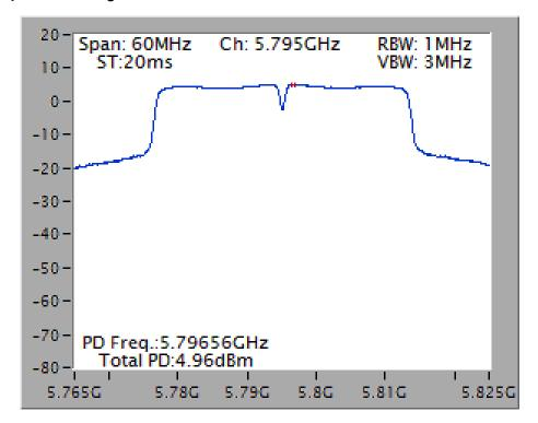
Power Density Plot on Configuration IEEE 802.11ac MCS0/Nss2 VHT80 / Chain 1 + Chain 2 / 5775 MHz
