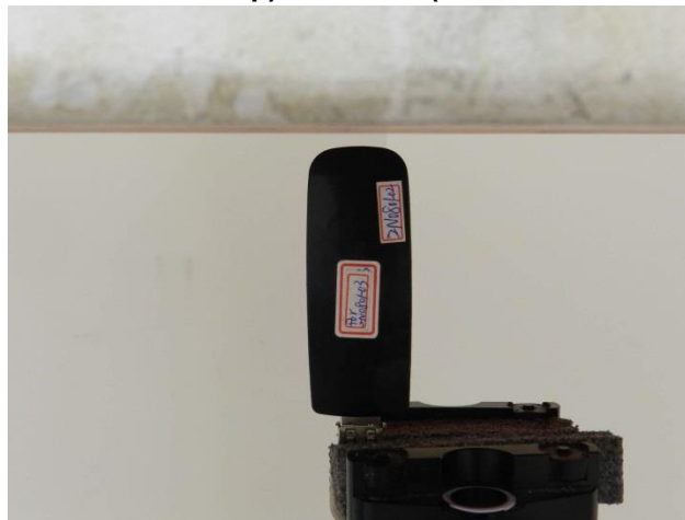
Direct Laptop Plug-in for USB Configuration 5 (Tip Mode with Phantom 5 mm Gap)
