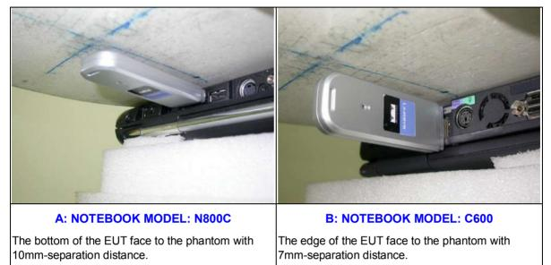
**NOTE:** The bottom of the notebook contacts the bottom of the flat phantom with 0mm-separation distance.
