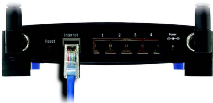
Figure 4-5: Connecting Another Router
