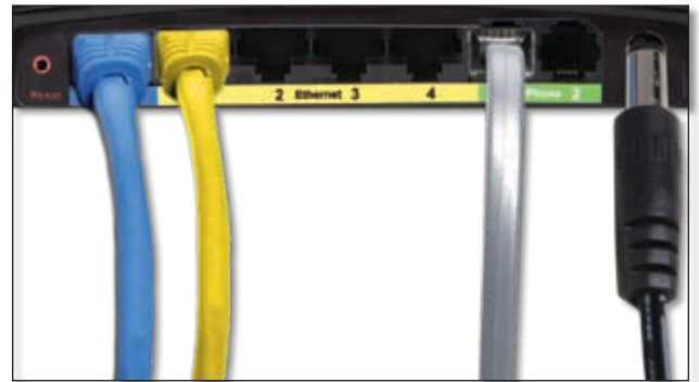
Connecting the Power Adapter
