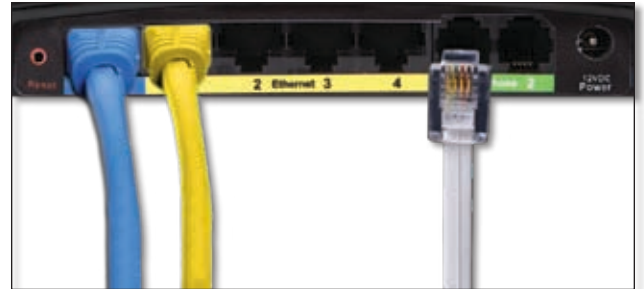
Connecting the RJ-11 cable
