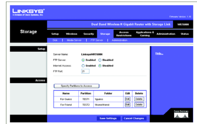
Figure 5-30: Storage Tab - FTP Server
