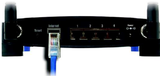
Figure 4-6: The Router with the Internet Connection is connected through the Internet Port
