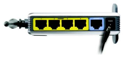
Figure 4-3: Connecting the Power
