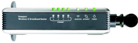
Figure 3-2: The Router's Front Panel
