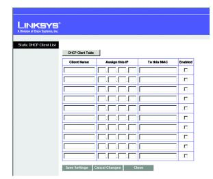
Figure 5-7: Static DHCP Client List
