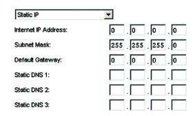
Figure 5-4: Static IP Connection Type
