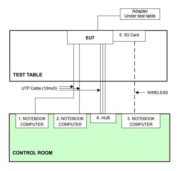
**NOTE:** 1. Support unit 1-4 were kept in the control room during the test.
