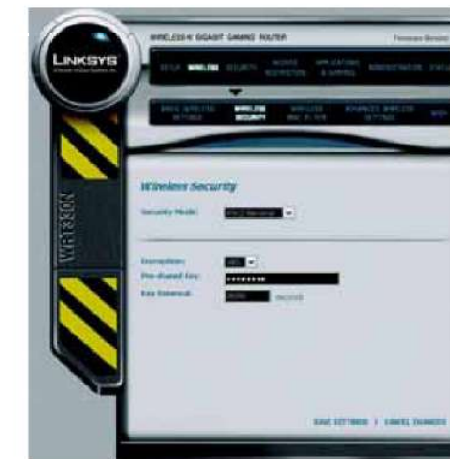
Figure 5-18: WIRELESS Tab - WIRELESS SECURITY - PSK2 Personal
