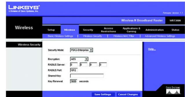
Figure 5-18: Wireless Security - PSK2-Enterprise
