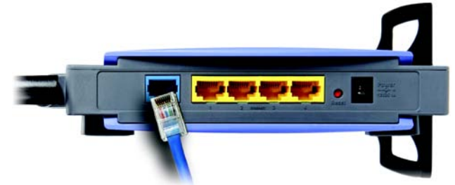
Figure 4-1: Connect the Modem
