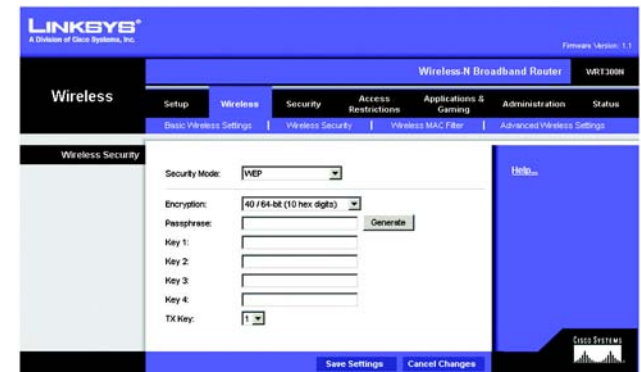
Figure 5-20: Wireless Security - WEP
