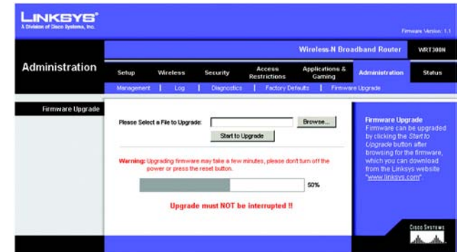
Figure 5-47: Administration Tab - Firmware Upgrade
