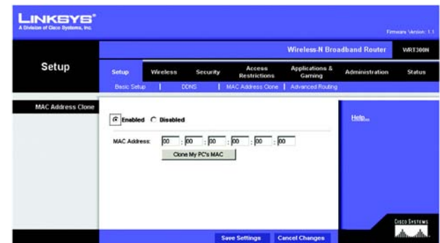
Figure E-5: MAC Address Cloning
