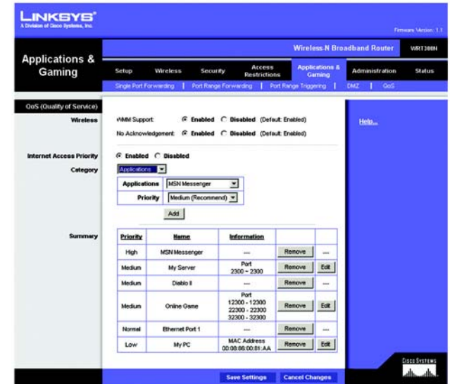
Figure 5-34: Applications & Gaming Tab - QoS (Applications)
