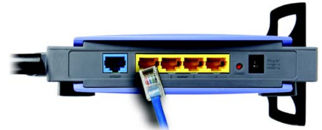
Figure 4-2: Connect a PC
