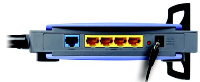
Figure 4-3: Connect the Power
