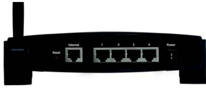
Figure 3-1: The Broadband Router's Back Panel
