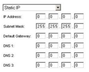
Figure 5-3: Static IP Connection Type
