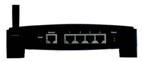
Figure 3-1: The Broadband Router's Back Panel
